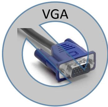
The old analog VGA cable has been replaced with an HDMI cable. HDMI carries both video and audio in the same cable.
