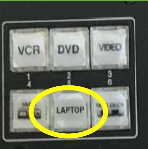
STEP 3. Make a selection from the input options. *Even if the desired input button is lit up,* please press the button. Please allow 3-10 seconds for image to appear.
