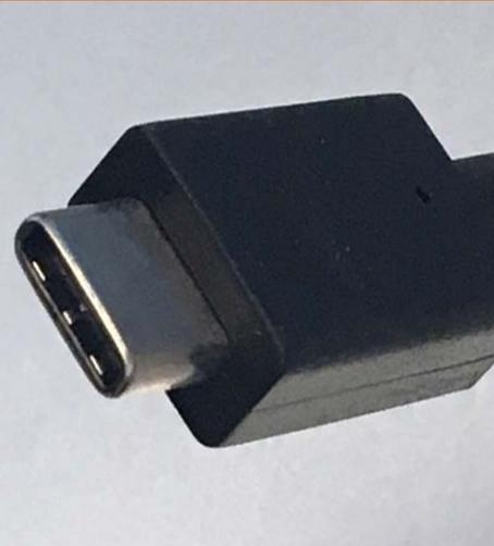
USB C: This connection carries audio, video and power over a single cable. Although fairly new, this connection is already being used in many devices, including the newest Macbook Pro laptops.
