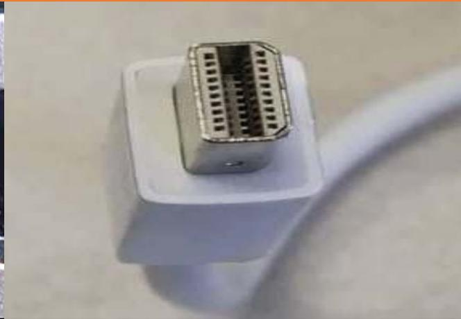
Mini Displayport to HDMI: This adapter is used on many devices, including multiple generations of Apple laptops, and the Surface Pro tablet. The adapter carries both audio and video signals.
