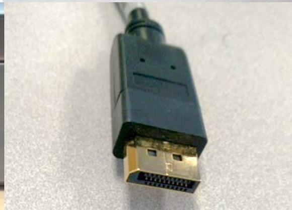
Display Port: This connection carries audio and video over a single cable. This connection can be differentiated from the HDMI connection by noting the flat vertical edge on one side of the connection.
